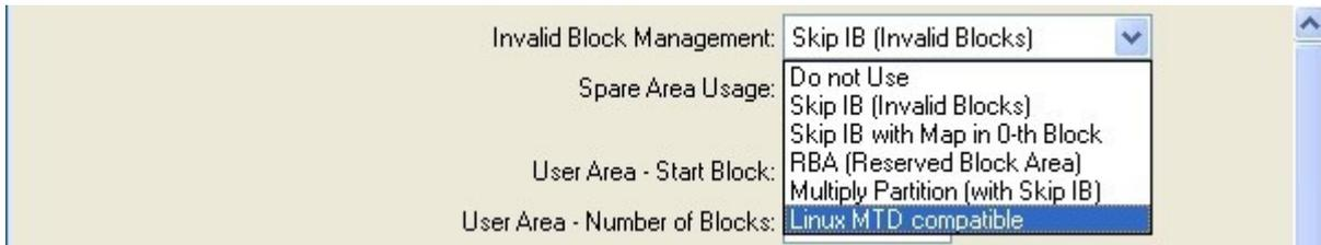
Figure 1. Enabling Linux MTD compatible feature
