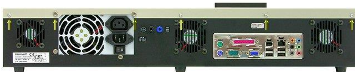
Figure 1 The screws position on the rear side of the programmer's unit
