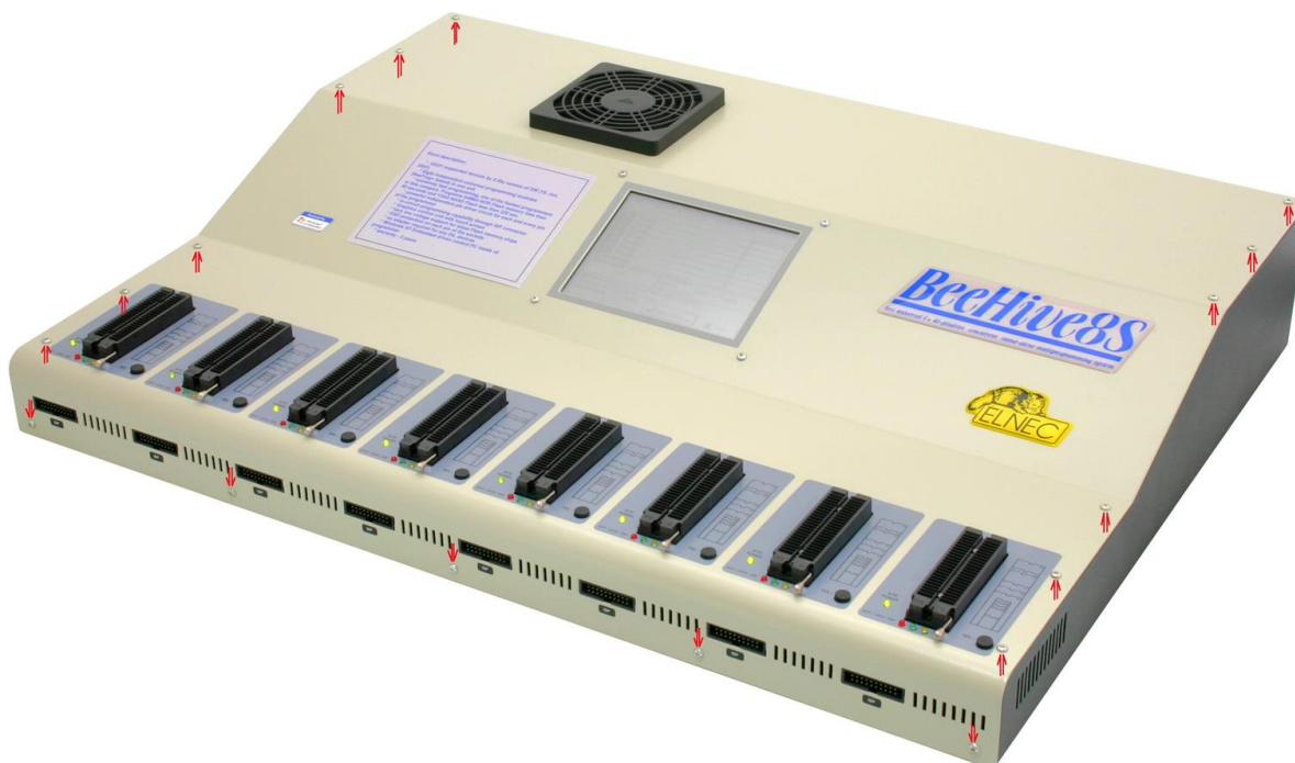
Figure 2 The screws position on the front and top sides of the programmer's unit
