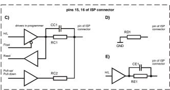
RA1 180R, RA2 1k3, RA3 22k, RB1 10k, RB2 10k, CC1 1n, RC1 1k3, RC2 22k, RD1 22k, CE1 1n, RE1 1k3,
