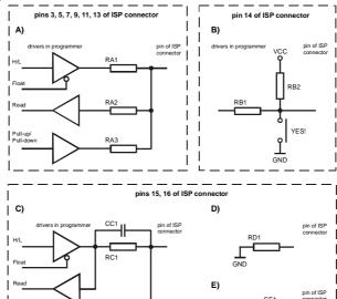
RA1 180R, RA2 1k3, RA3 22k, RB1 10k, RB2 10k, CC1 1n, RC1 1k3, RC2 22k, RD1 22k, CE1 1n, RE1 1k3,
